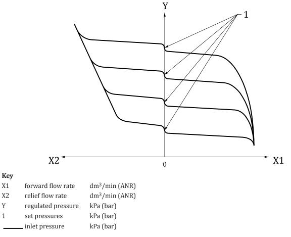
NOTE <u>Figure 2</u> is only an example of flow rate-pressure characteristic curves. For some components, the several flow- pressure curves do not terminate at the same point at maximum forward flow rate.
