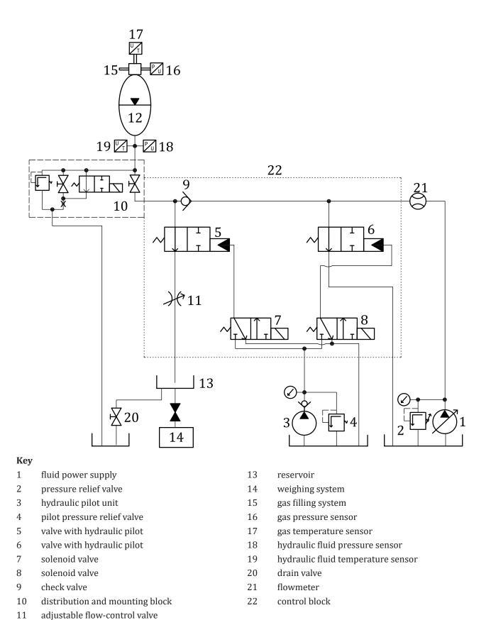
Figure E.1 — Example of hydraulic schematic diagram of an accumulator test bench
