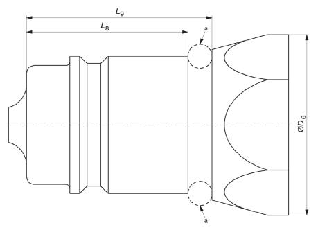
Shape of neck between  $L_8$  and  $L_9$  is optional but shall be circular to accommodate dust sealing. а
